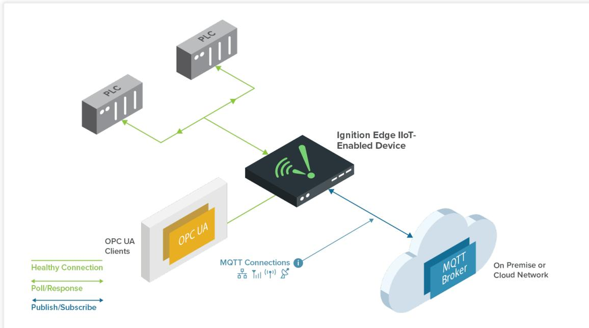
**Ignition Edge IIoT Standalone:** Use Edge IIoT as a standalone edge gateway to publish device data from the edge of the network to an MQTT broker.
