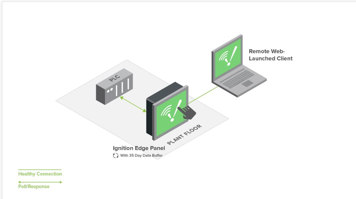
**Standalone HMI:** Use Ignition Edge Panel to create a standalone HMI at the edge of the network.
