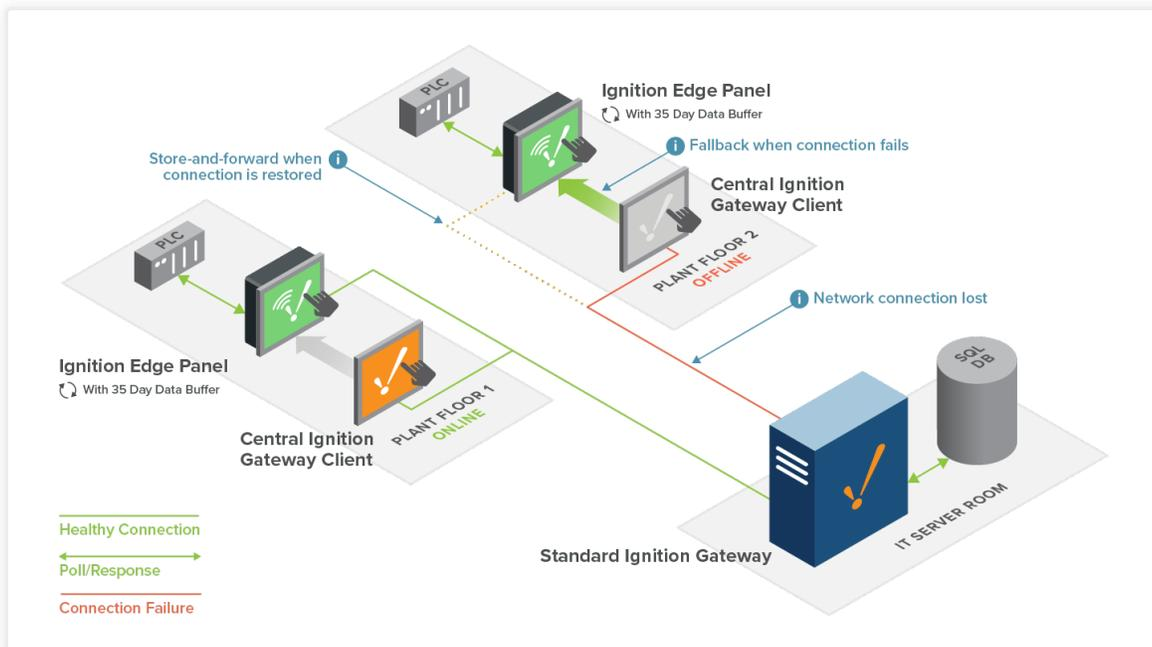
**Hub-and-Spoke with Local Client Fallback:** Use Edge Panel to add local client fallback to a hub-and-spoke architecture. Edge Panel provides visualization at the edge, a 35 day data buffer to cache PLC data while a network connection is down, and store and forward functionality for when the connection is restored.
